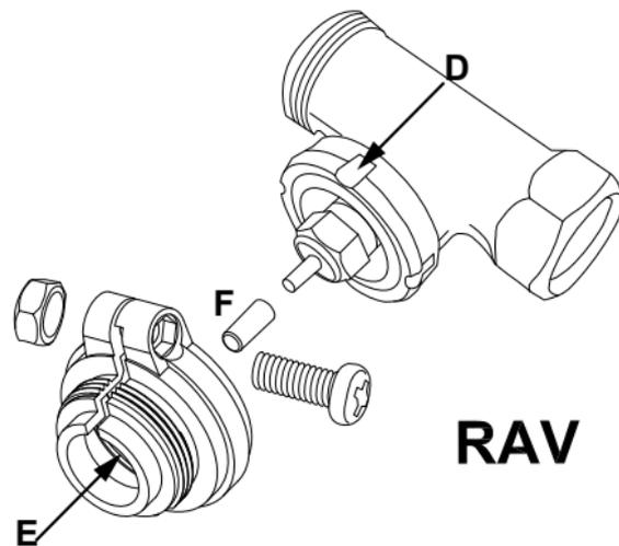
**i** During installation, please ensure that the pins inside the adapter (E) are lined up with the notches (D) on the valve. Ensure that a suitable adapter for the valve is properly clipped on.
