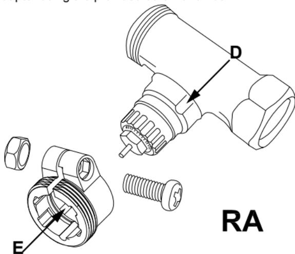
**i** During installation, please ensure that the pins inside the adapter (E) are lined up with the notches (D) on the valve. Ensure that a suitable adapter for the valve is properly clipped on.
